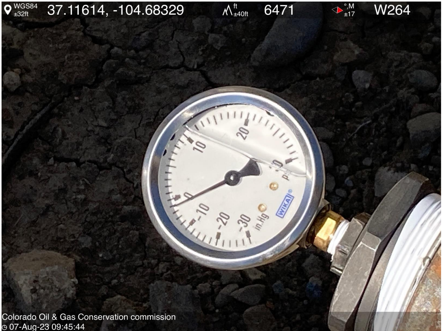
PHOTO 6: T-C PRESSURE -2, PRESSURE EQUALIZED IN 3 SECONDS. PRESSURE STAYED ON 0 FOR 15 MIN.
