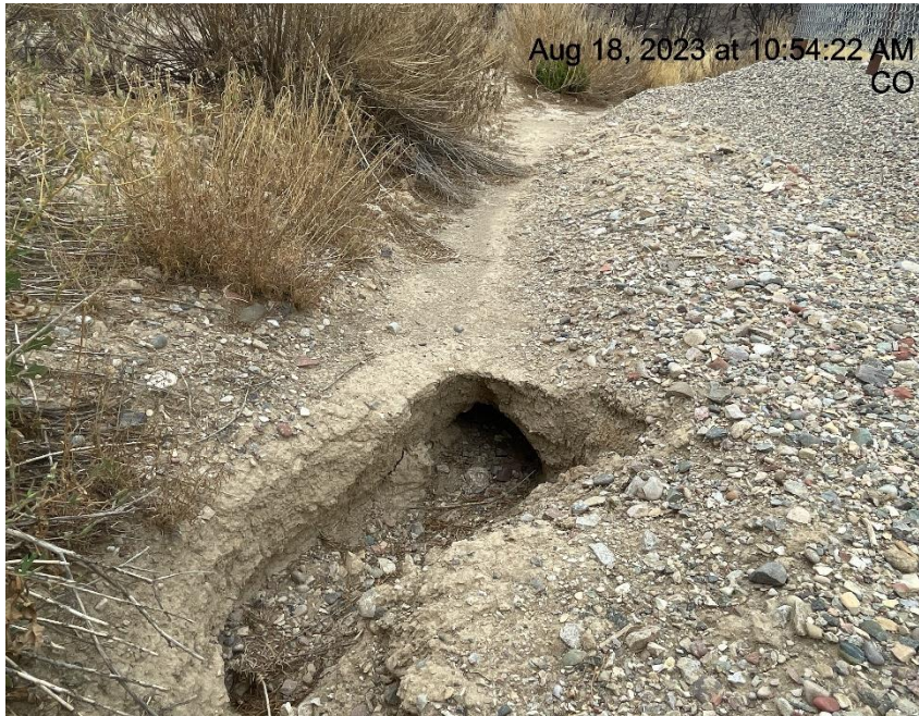
Photo # 6419 Erosion/tunnel erosion (NE corner of location)
