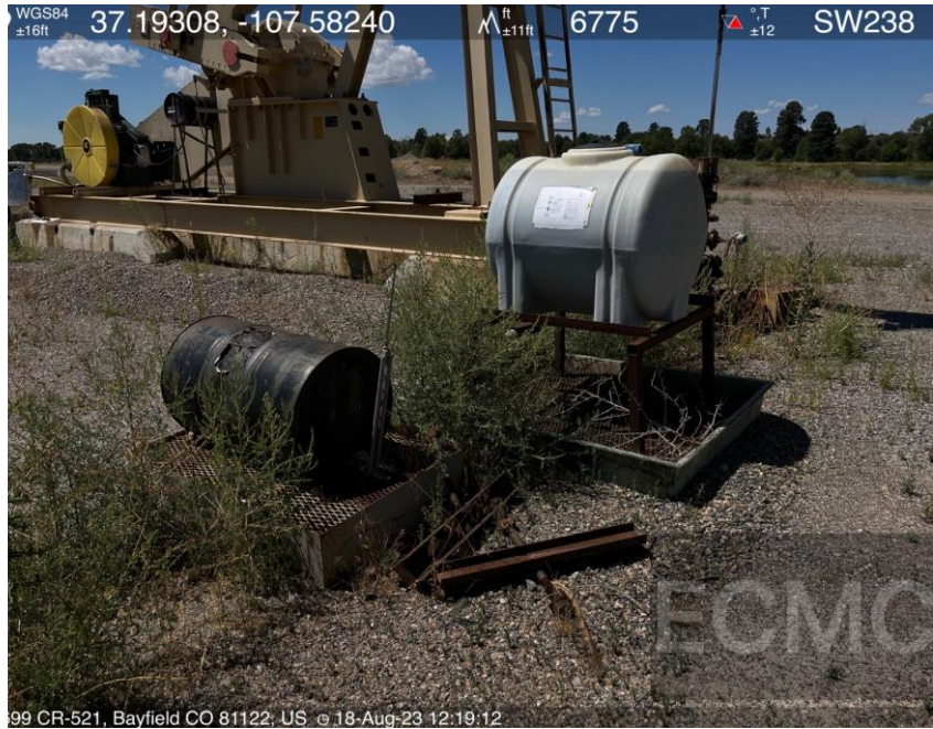
Photo #1. Disconnected, flammable materials stored near wellhead.
