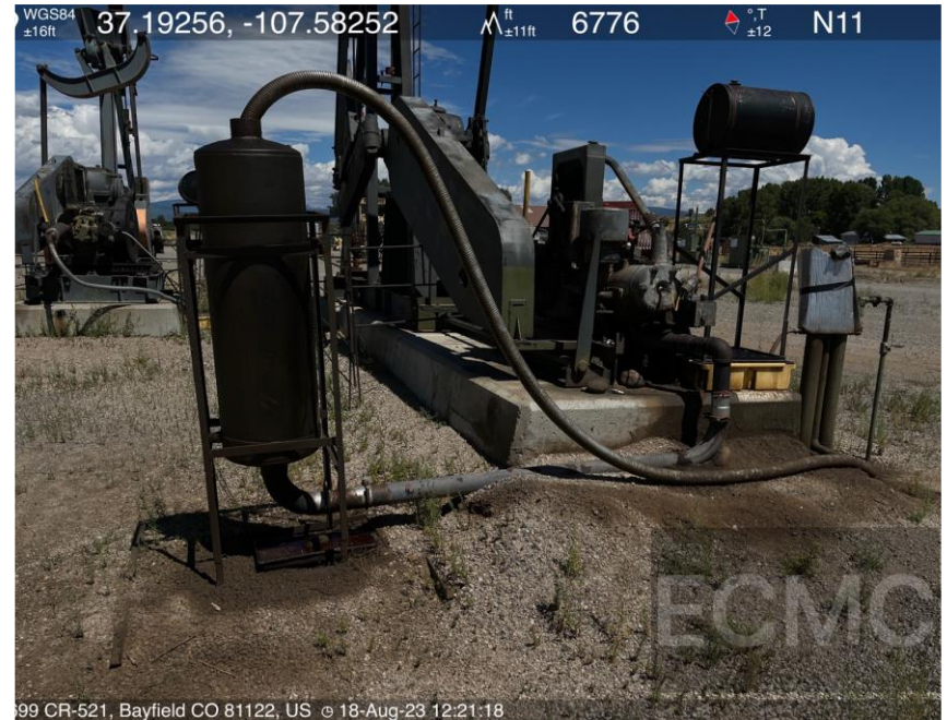
Photo #4. Impacted material on ground around prime mover.
