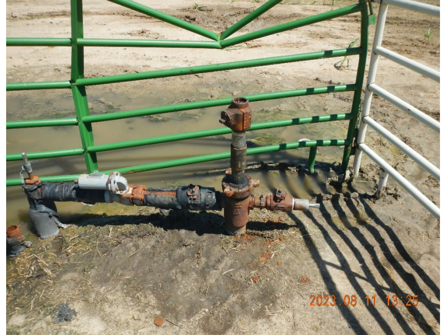
2. View of repaired Wellhead with bent tubing joint removed.
