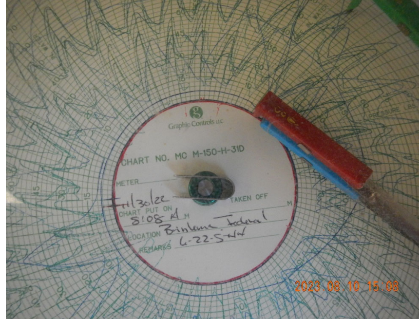
6. View of Chart inside Meter Box at time of inspection.
