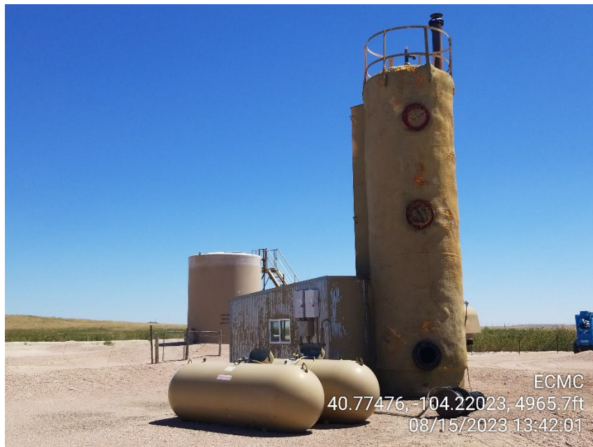
Photo 3 – Heater Treater and Propane Tanks
