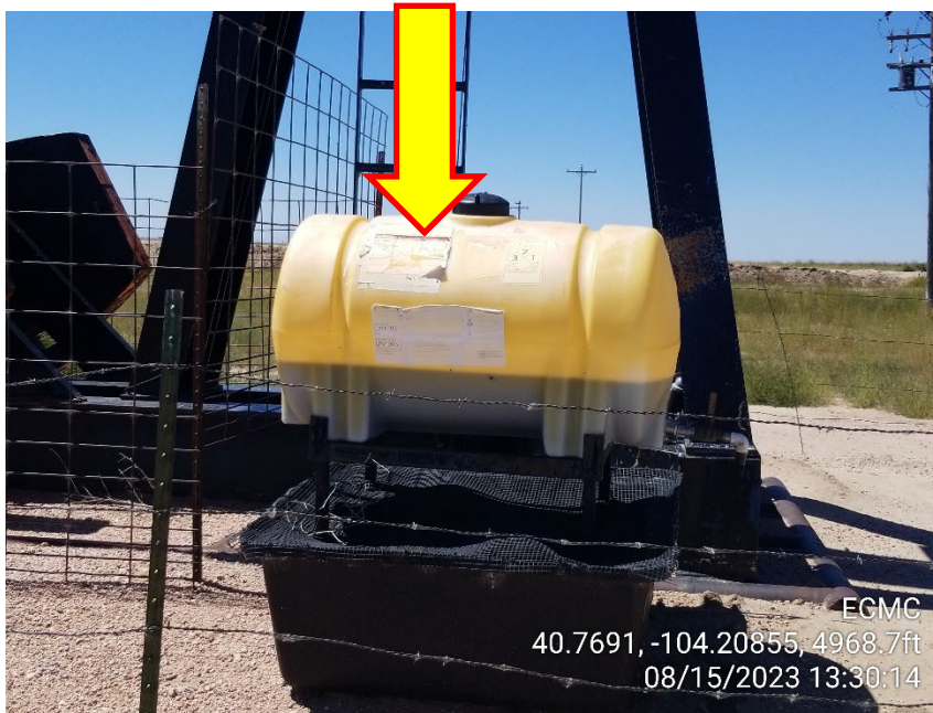
Photo 3 – Labels have faded no longer visible
