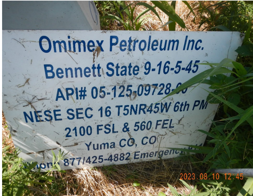
1. Well sign broken out of bracket. Note vegetation.
