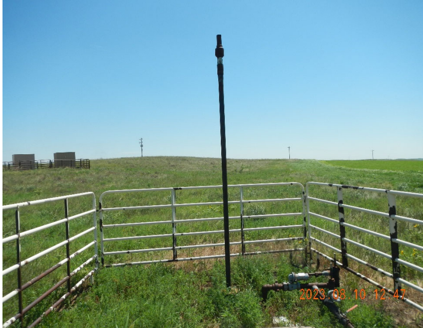
3. View of Wellhead with tubing approximately 12' out of well cap. Note vegetation.
