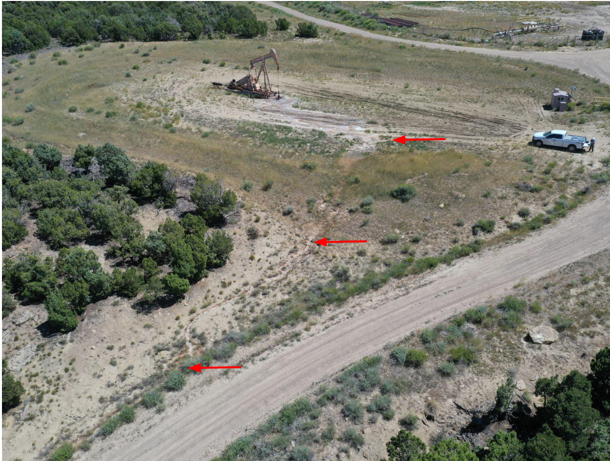
Photo 4: Photo taken with a sUAS. Photo shows that a spill/release of E&P waste fluids originating at the wellhead has impacted large areas of the Location and traveled off-site to the northwest along and on the lease road (red arrows); spill traveled approximately 1,000 feet from point of release to approximate end point.
