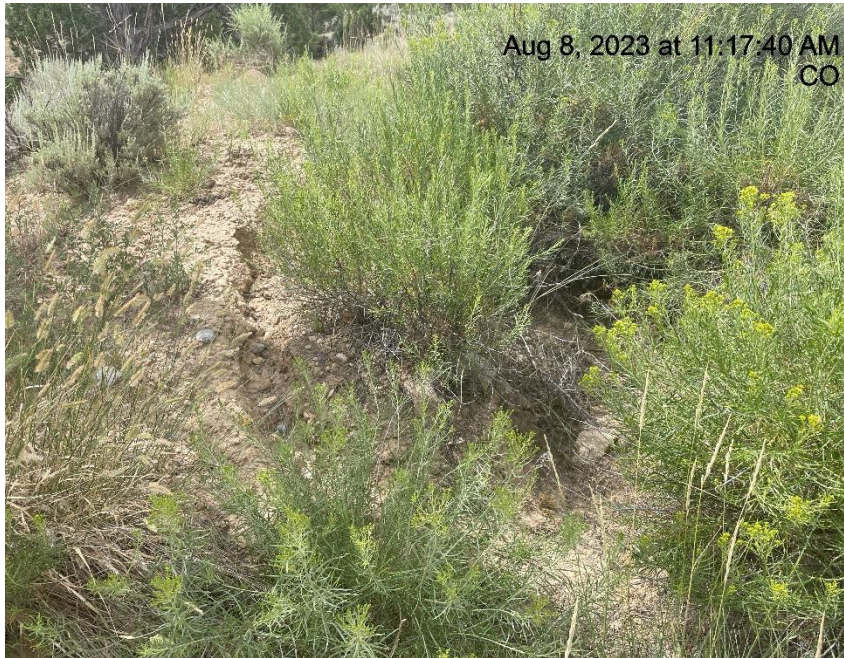
Photo # 5305 Erosion & transport of sediment (East edge of location near tank battery)
