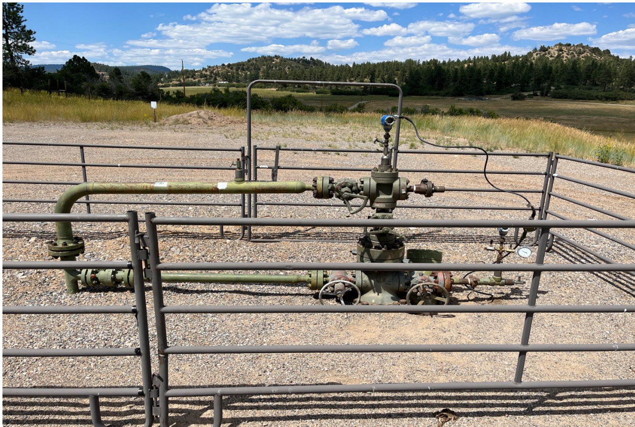
Photo #2. View of the wellhead assembly.
