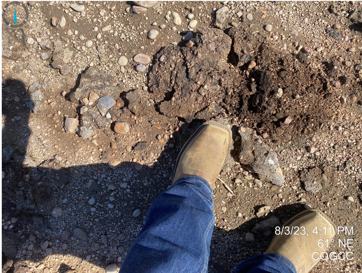
Photo 4. Continued from Photo 3. Close up photo of stained material (a chemical odor from the soil was detected during this inspection).
