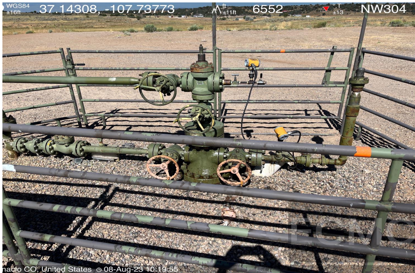
Photo #3. View of the #4 wellhead assembly.
