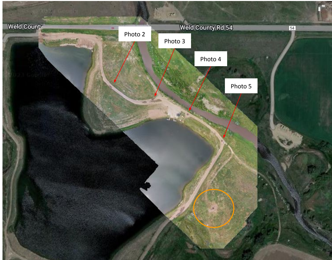
Photo 1. Drone aerial imagery illustrates the access road which has been used for the Croissant 30-12, 30-13 and Betz 30-15 well locations. Red arrows indicate road damages from plugging operations on Betz 30-15 (orange circle).
