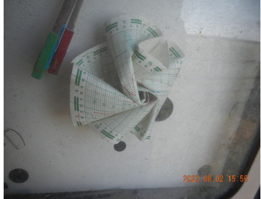
10 Chart has twisted inside the unchecked Meter Box.
