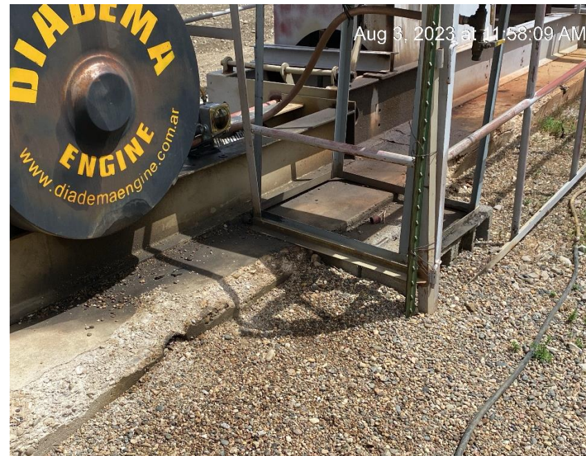
Equipment leaks. Stained soil
