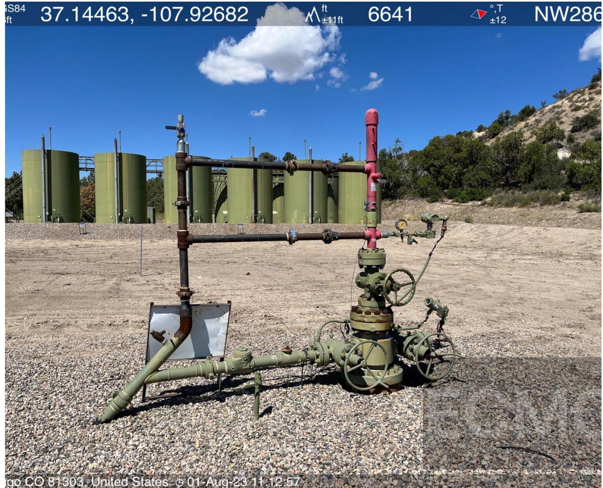
Photo #2 View of the wellhead assembly.
