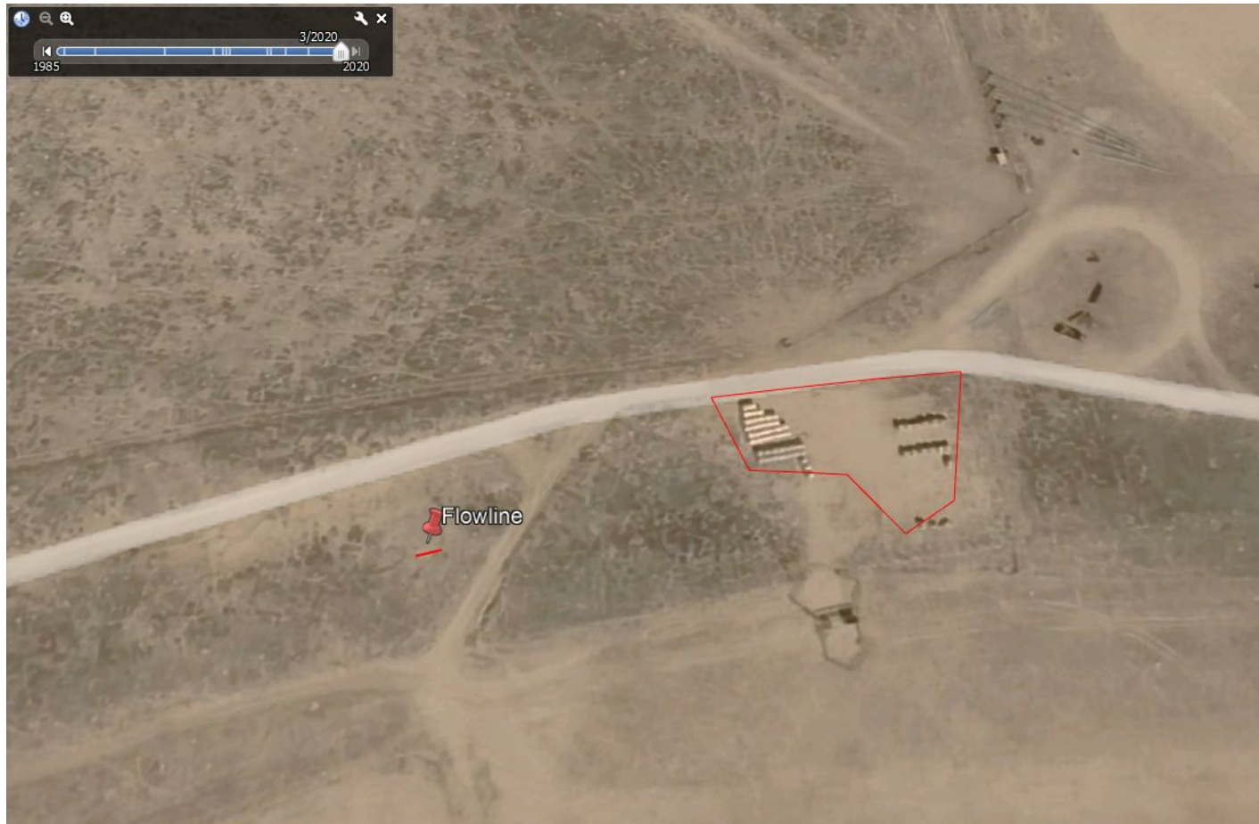
Photo 6. Google Earth aerial imagery taken circa 03/2020, illustrating that the former tank battery location does not appear reflective of adjacent reference areas as it is being used as storage. The tank battery location will need to be reclaimed per Rule 1004 standards.
