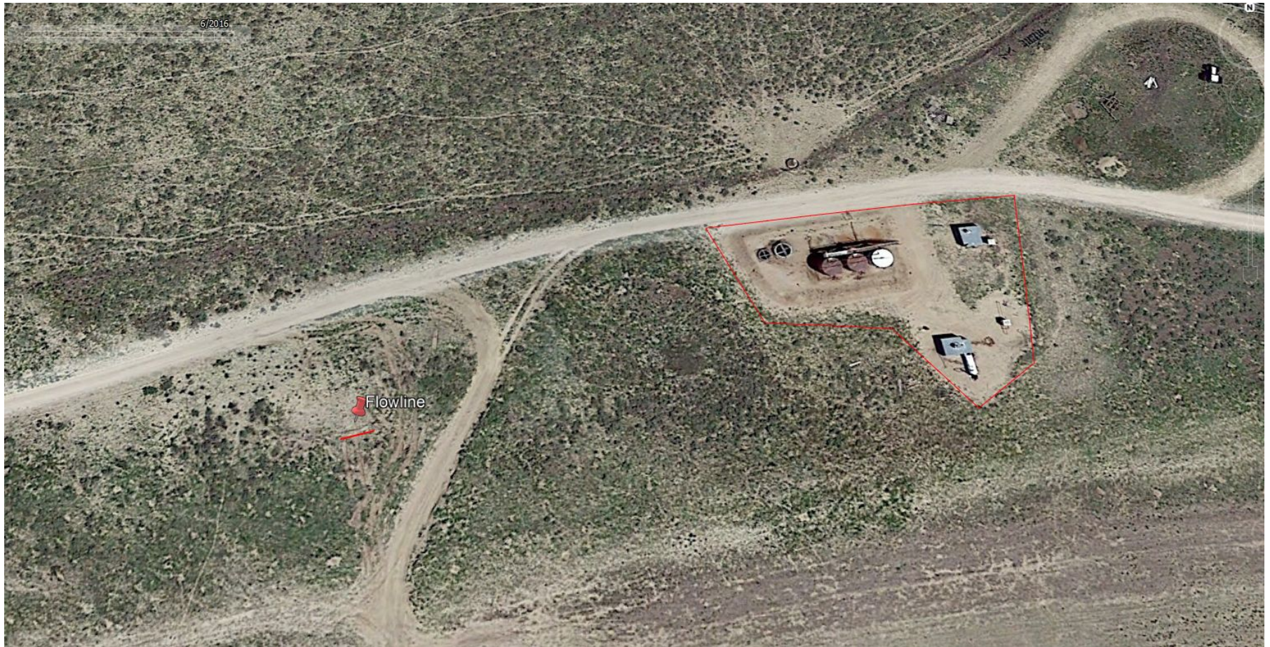
Photo 5. Google Earth aerial imagery taken circa 06/2016 illustrates the flowline position and the former tank battery location.
