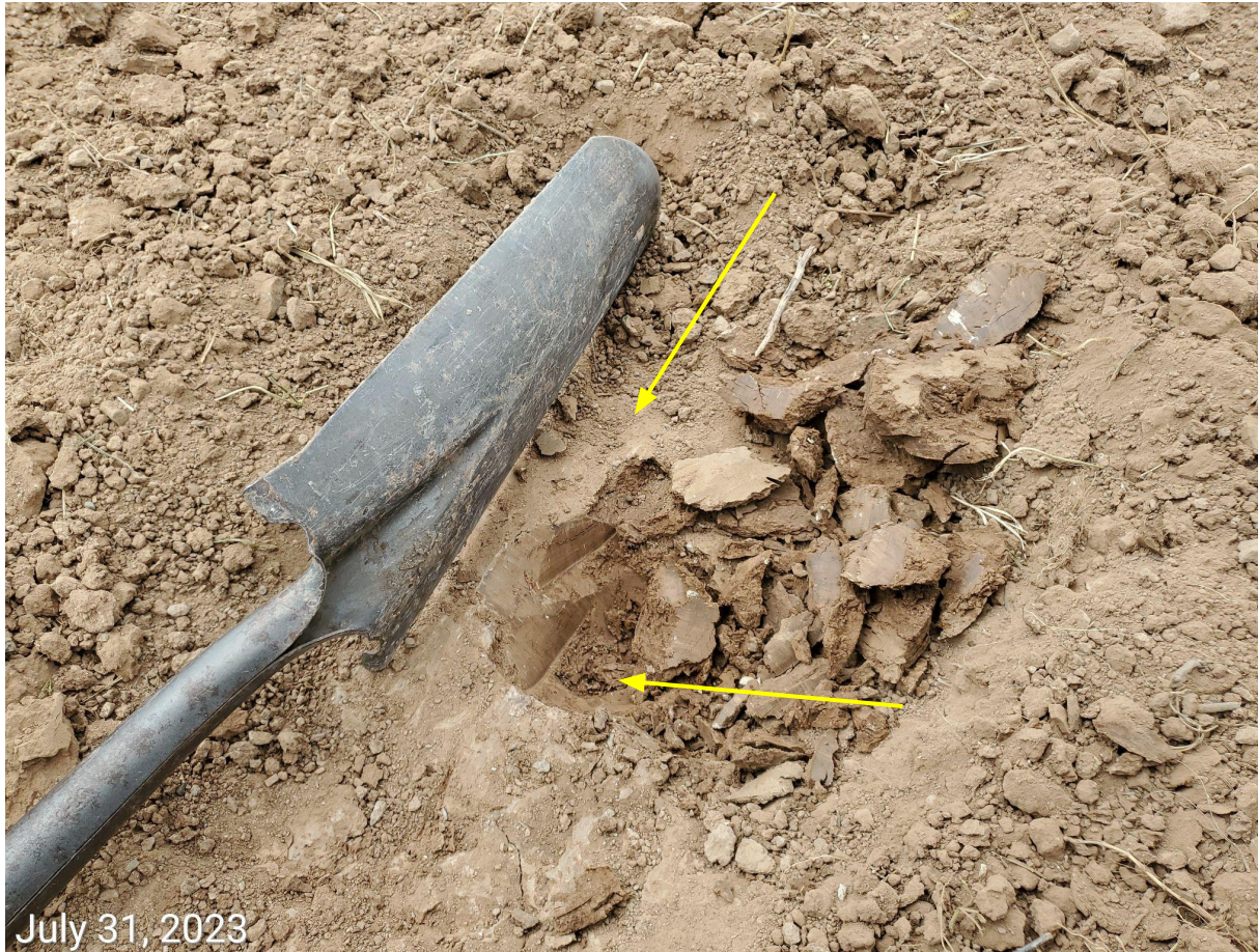
Photo 4: Photo shows compaction alleviation test-pit performed by Reclamation Specialist on the Location. Photo shows an apparent zone of compaction ~2-4 inches below the soil surface.
