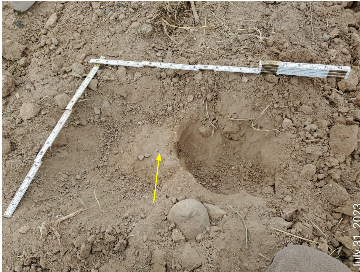
Photo 8: Photo shows compaction alleviation test-pit performed by Reclamation Specialist on the access road. Operator appears to have ripped a section of the access road in one direction. Photo shows an apparent zone of compaction remaining at road
