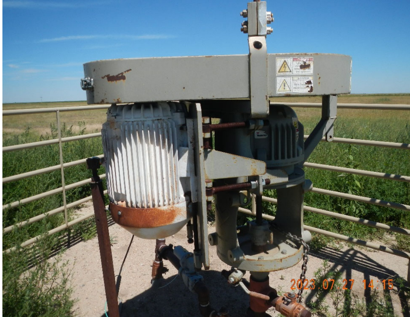
3. Progressive Cavity on Wellhead.
