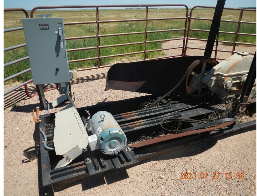
4. View of Prime Mover with drive belts disconnected.
