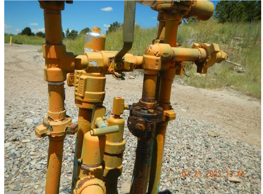
At group of unused flowlines north of the tank battery, a line with a leaky valve was saturated with condensate and stained ground.
