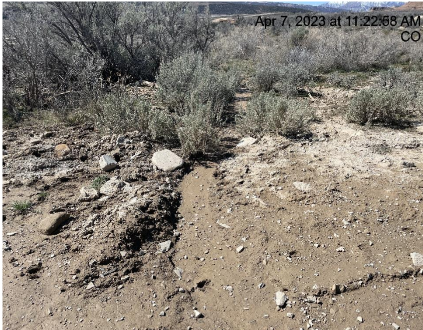
Photo # 4639 From Inspection 708900241 conducted on 04/07/2023 Erosion & transport of sediment off lease road/insufficient BMP's
