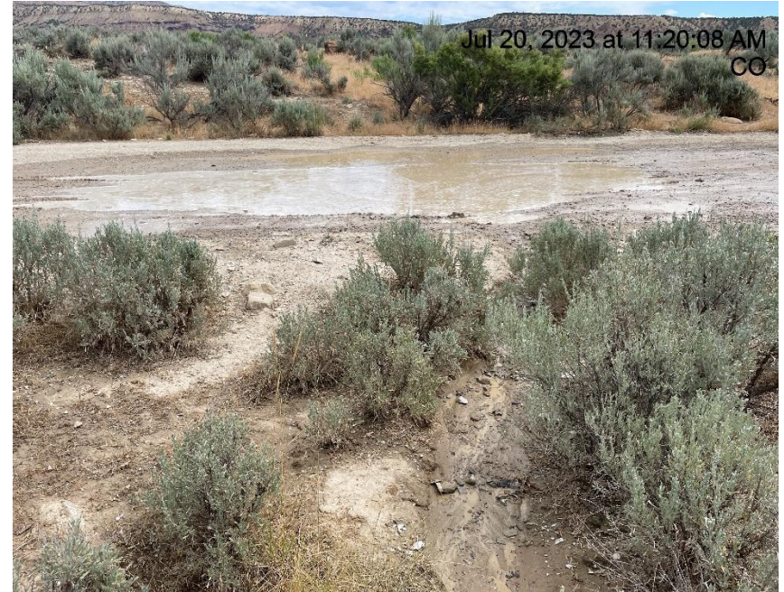
Photo # 3495 Erosion & transport of sediment off lease road/insufficient BMP's
