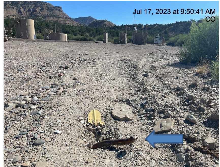
Photo # 3155 Debris/Hazard – same broken deadman /anchor sticking up out of the ground from a different angle
