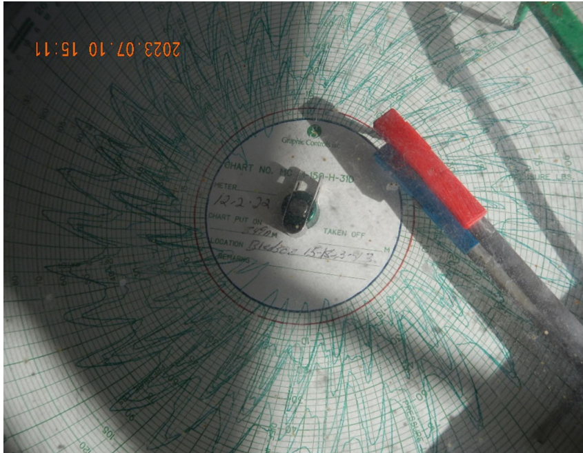
11. View of Chart dated 12-2-22 that was in Meter Box at time of inspection.
