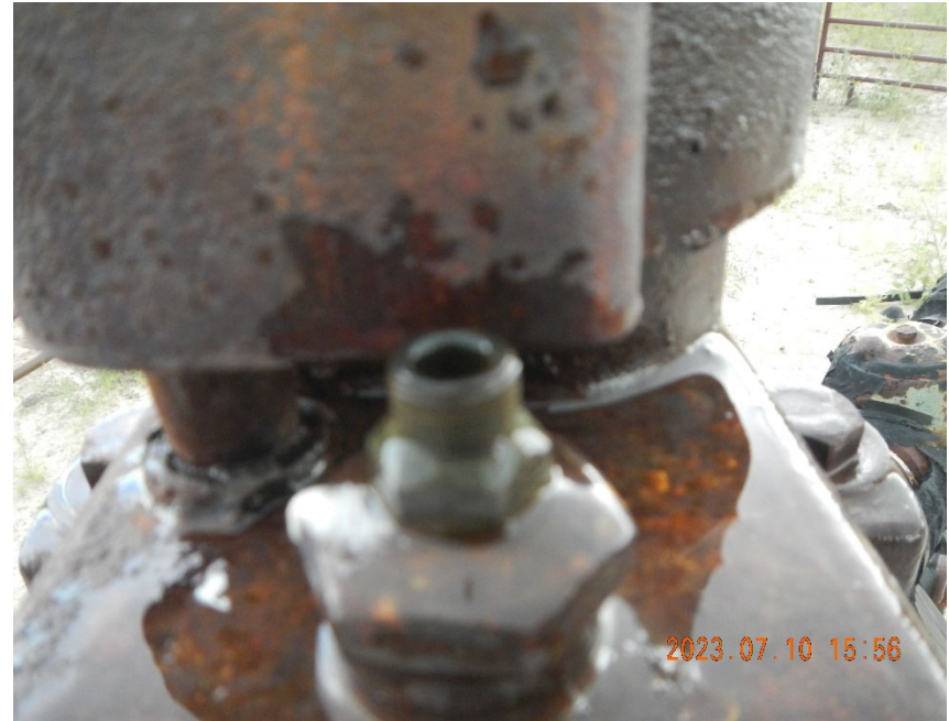
10. Gas is venting through Compression Bolt.
