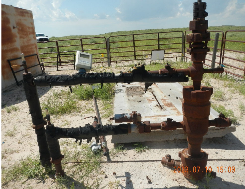
3. Closer view of wellhead. Concrete Pumping Unit Slab in the background.
