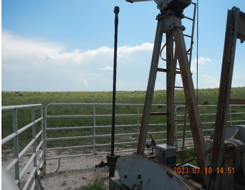
3. Tubing appears to be pulled above well and Ball Valve at top.
