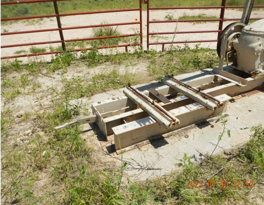
7. Prime Mover has been removed from Pump Jack. Note surrounding vegetation growth.
