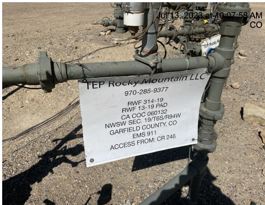
Photo # 2920 Wellhead sign missing API #
