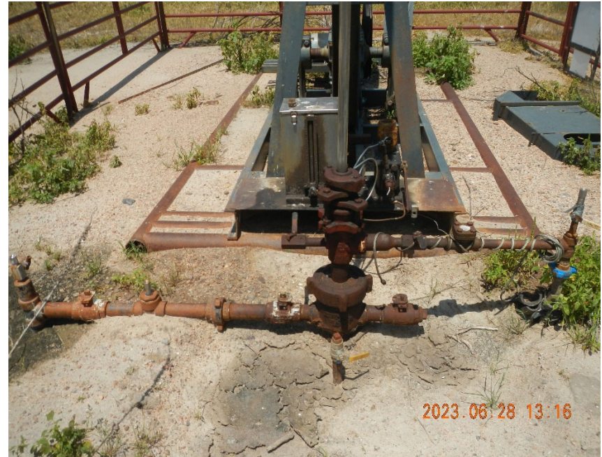
2. View of wellhead. Note stained soils in lower left of picture.
