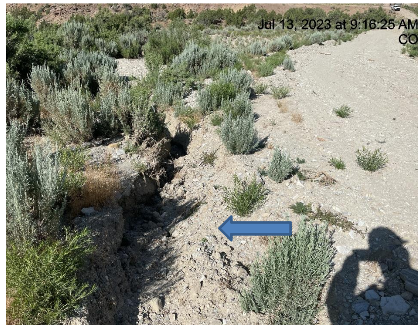
Photo # 2891 Erosion & transport of sediment (edge of lease road, approximately 1/10 th of a mile from location)
