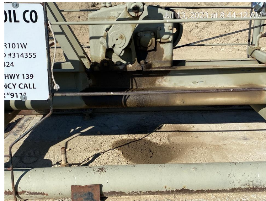
Oily waste on unit and wooden base
