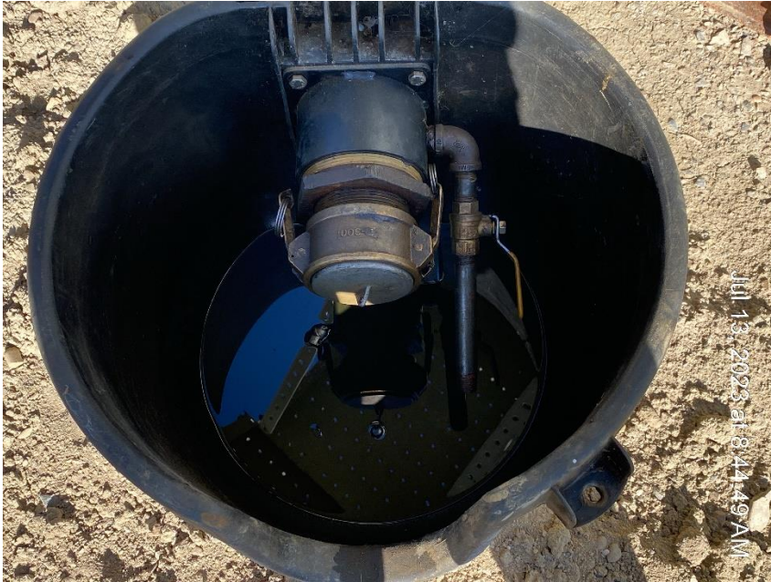
Valve open on loadline
