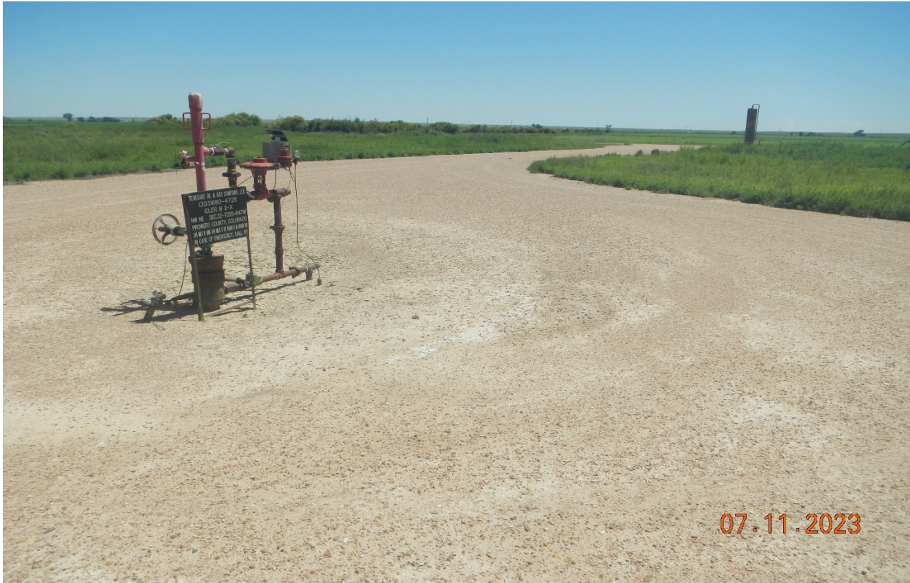
Photo 4. There is well sign posted at the wellhead. The well is a distance away from the tank battery and an addition sign should be posted at the tank battery.
