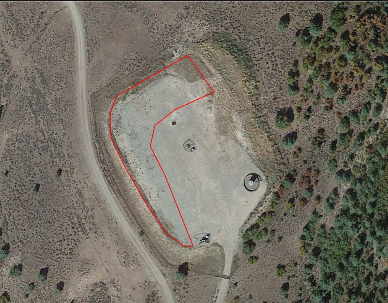
Photo 5: 2019 Google Earth aerial image of the Location. Polygon represents approximate areas of the Location not reasonably needed for production requiring work including, but not limited to, compaction alleviation, recontouring/regrading and reclamation.
