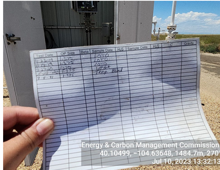
Photo 5: Gas meter not annually calibrated
