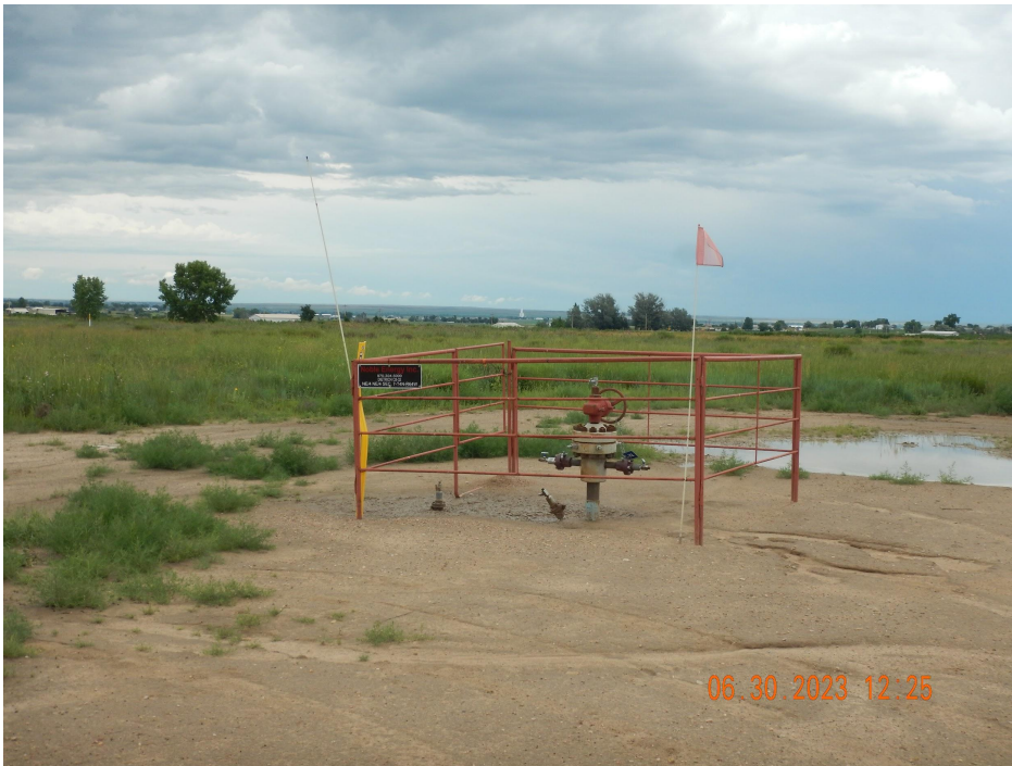
Photo 1. Photo taken from the well location, facing East. Photo illustrates Operator has plugged and abandoned 5 of the 6 wells.
