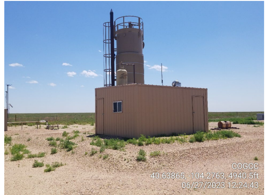
Photo 10 – Heater Treater
