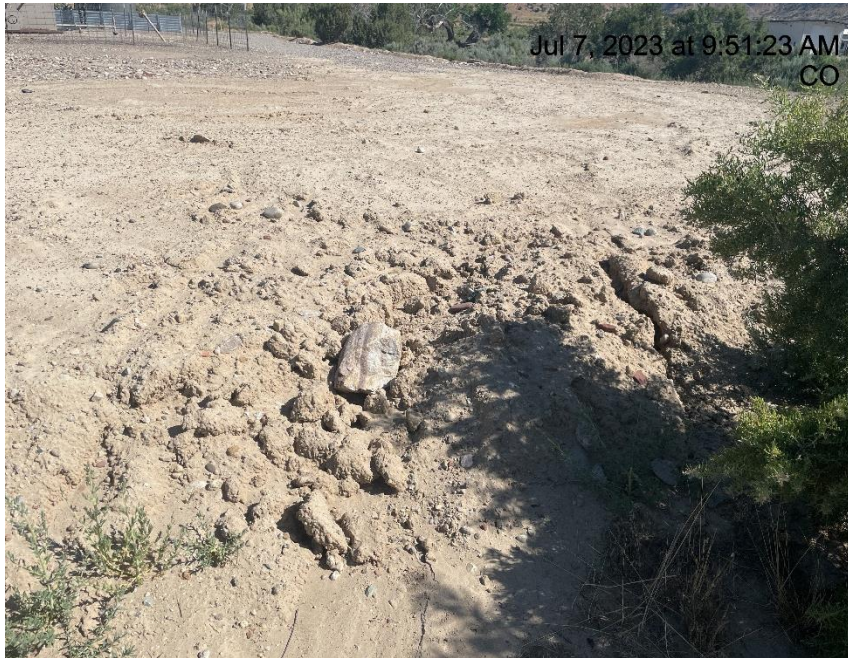
Photo # 2466 Erosion & transport of sediment off location & into vegetated area
