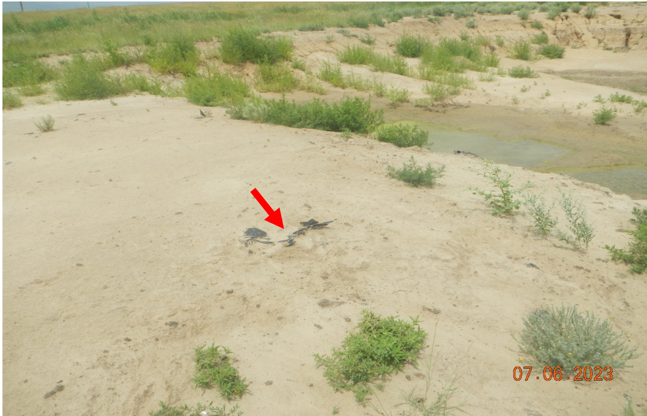
Photo 8. Facing southwest toward the area where the spill occurred. Remediation project: 20712. Some areas have been excavated more than other areas. There are still areas of impacted soils observed. Red arrow points to liner material and stained soil.
