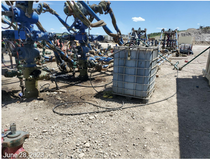
Photo 23: Photos examples showing containers on Location missing spill prevention/containment BMPs.
