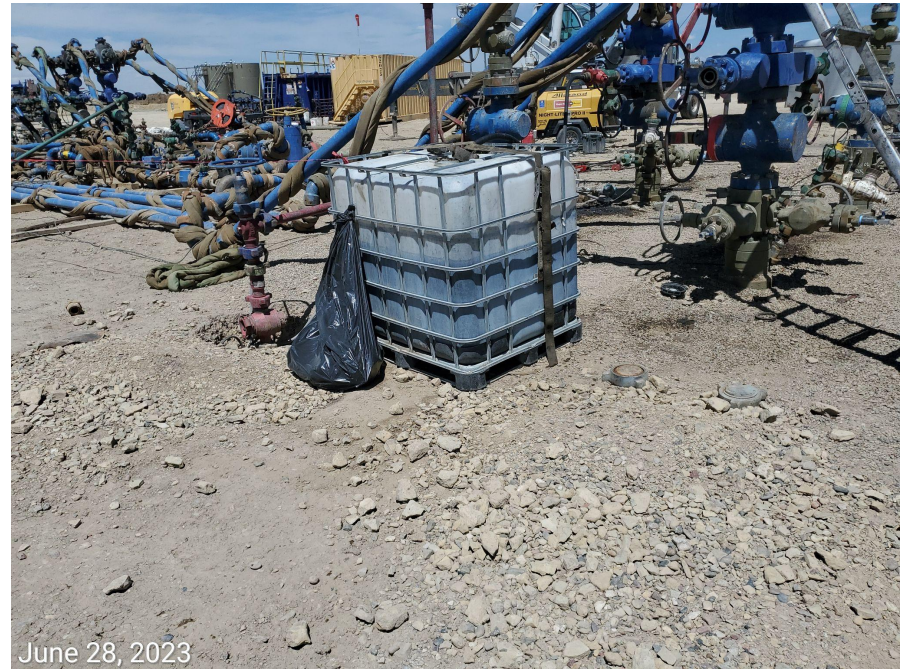
Photo 23: Photos examples showing containers on Location missing spill prevention/containment BMPs.
