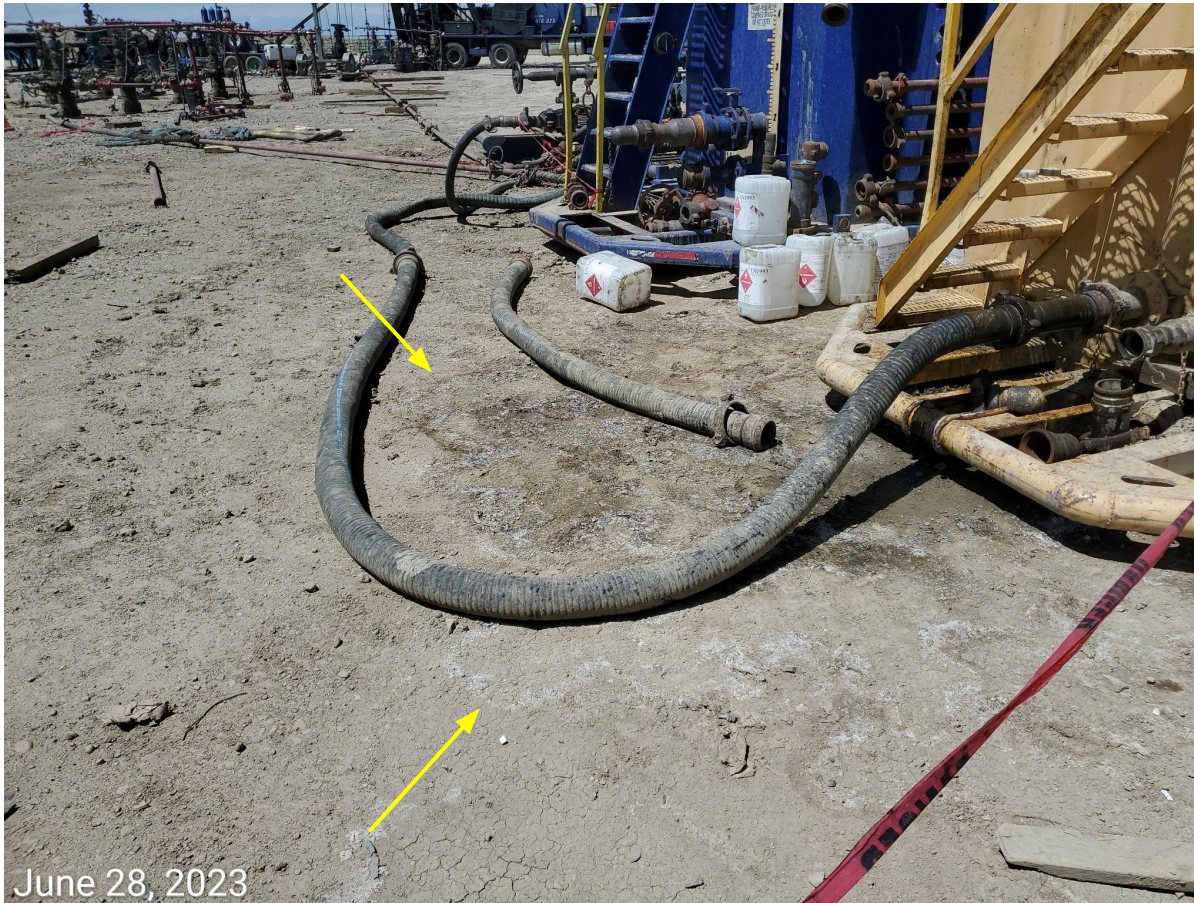
Photo 26: Photo shows stained soils from what appears to be a spill at the tank. See comments under photo 12 regarding tank labeling, trash, and spill prevention/containment BMPs.
