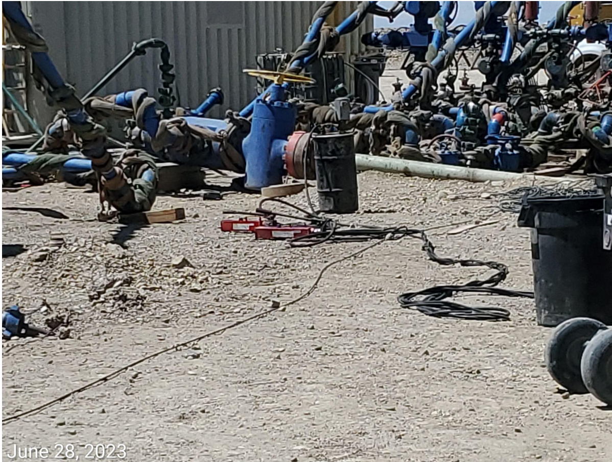
Photo 22: Photo example showing barrel observed missing spill prevention/containment BMPs.
