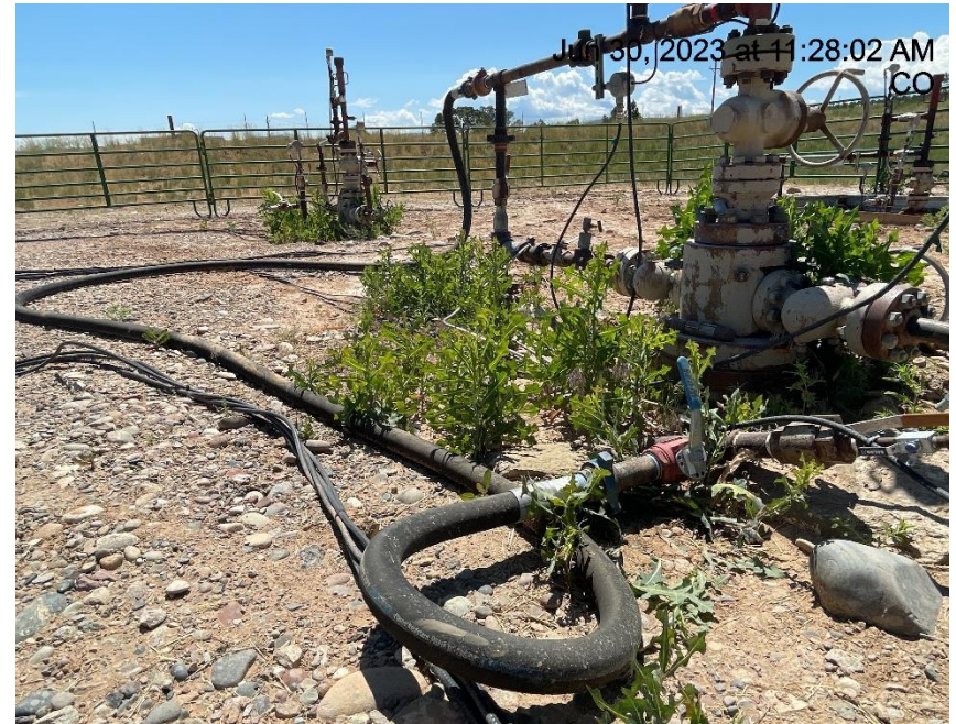
Photo # 2295 KELLY 34-13 well bradenhead connected to flowline, no check valve visible
