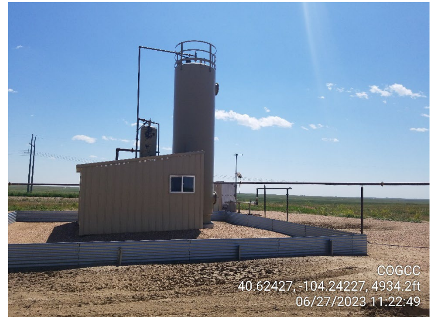
Photo 4 – Heater Treater
