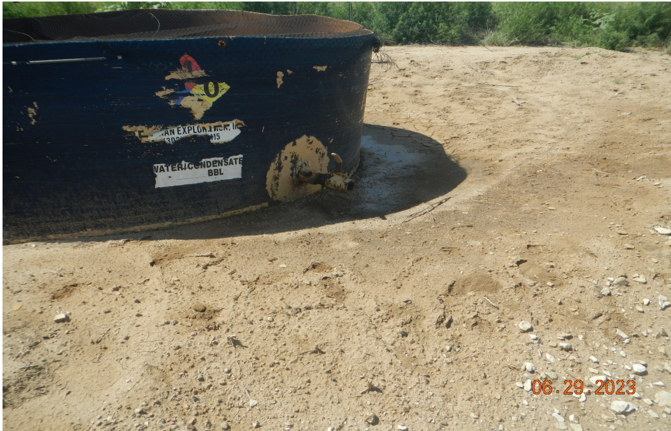
Photo 2. There is a dripping condensate leak at the valve of the tank. The berm around the tank is not sufficient to contain a spill. The labeling on the tank is degraded.
