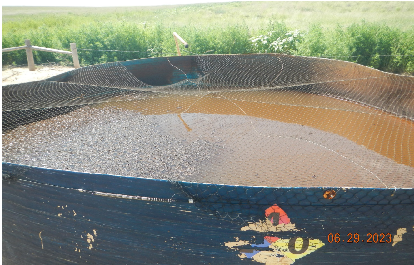
Photo 3. The netting on the open top tank is torn and needs repair.
