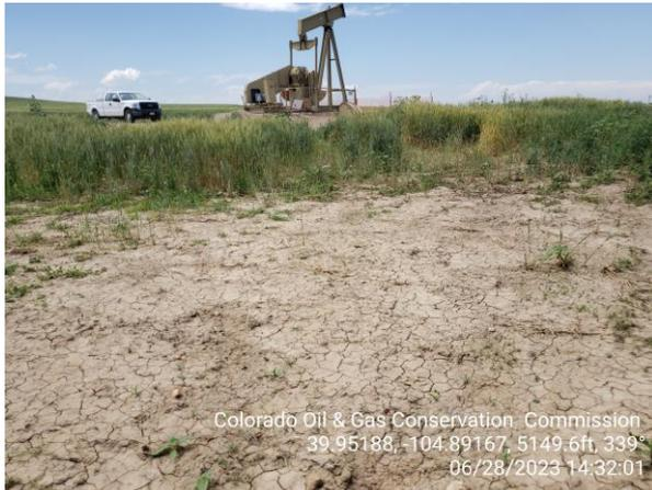
**Photo 7 No BMPs installed, sediment is running off the wellsite into the planted field towards the SE.**
