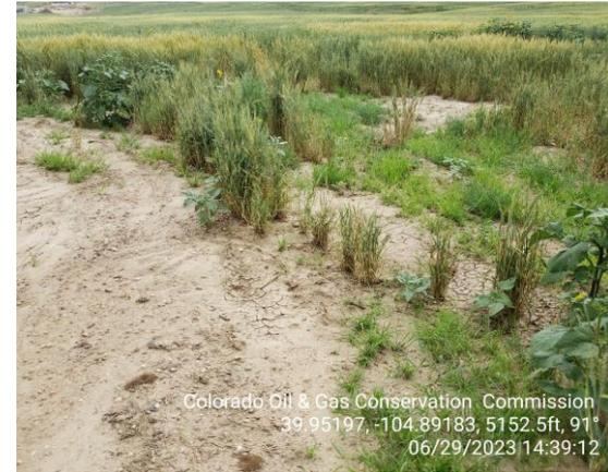
**Photo 23 Dirt/Sediment washing off the wellsite into the field.**
