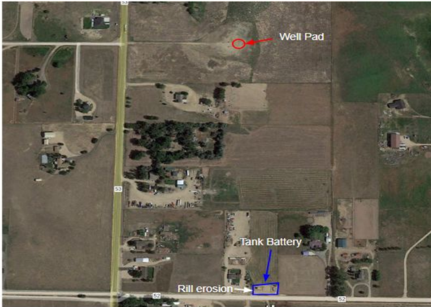
Photo 1. 2021 aerial imagery of the well pad (north is up). The tank battery highlighted in blue remains in service for the temporarily abandoned well API #123-11998.
