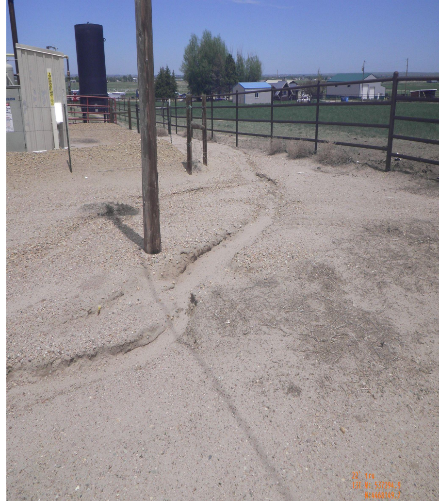
Photo 3. Rill erosion observed on the western edge of the tank battery has not been addressed since previous inspection form was submitted on November 16th, 2021.
