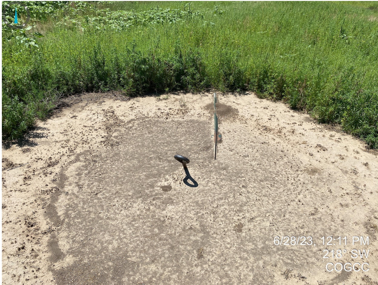
Photo 11. Guy line anchors not properly marked.
