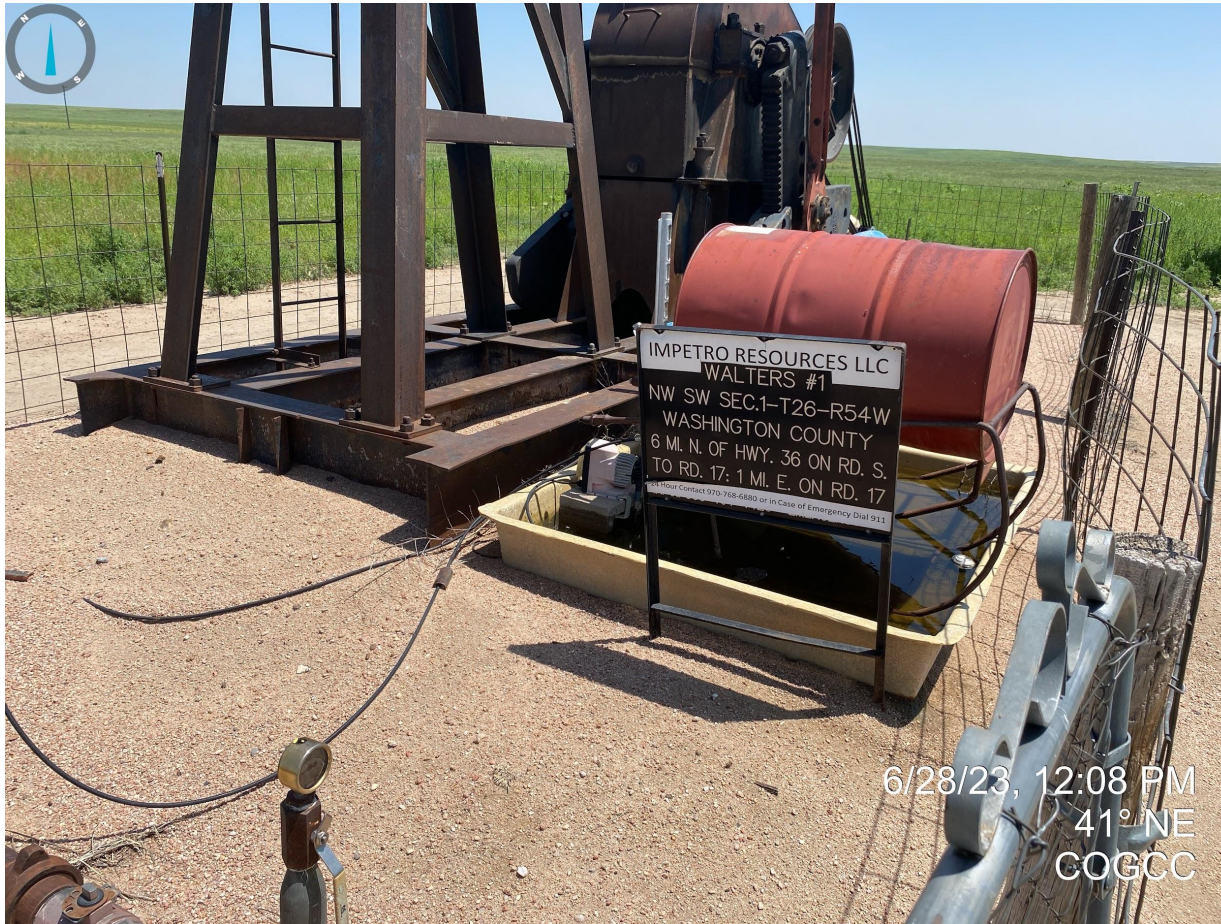
Photo 3. No wildlife protection equipment observed around secondary containment and tank labels are peeling, faded, cracked and/or not legible.
