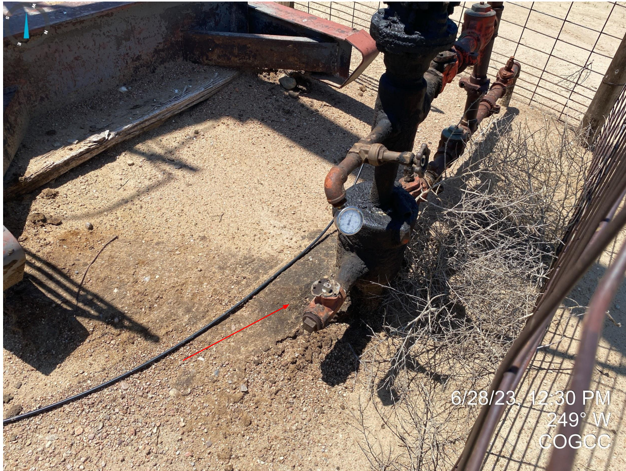
Photo 7. Stained soil around wellhead.
