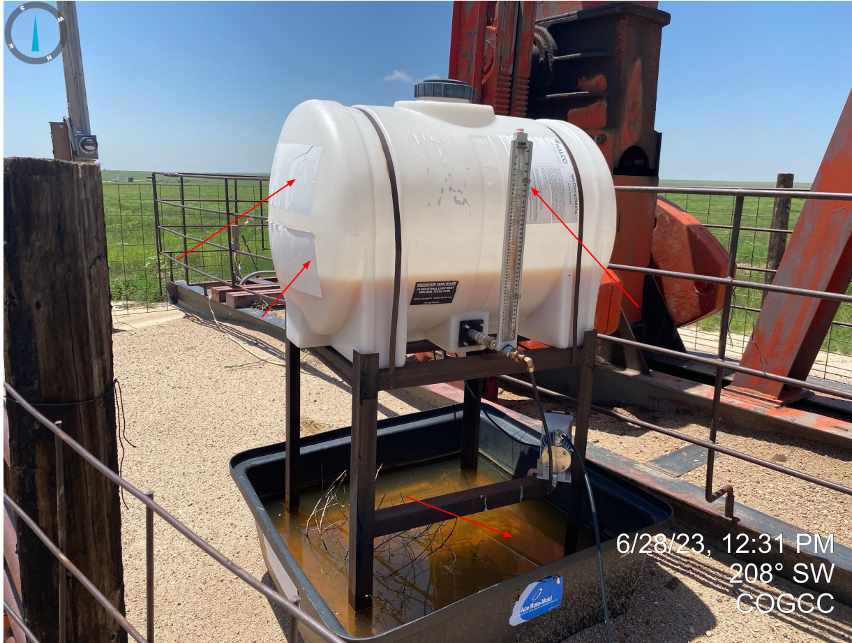
Photo 8. Day tank labels are not legible and missing wildlife protection equipment.
