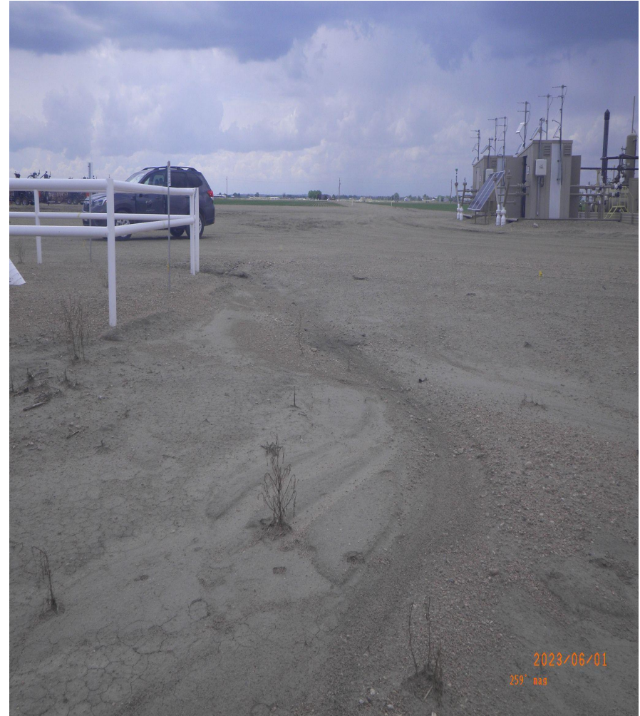
Photo 3. Rill erosion located on south eastern edge of the tank battery.
