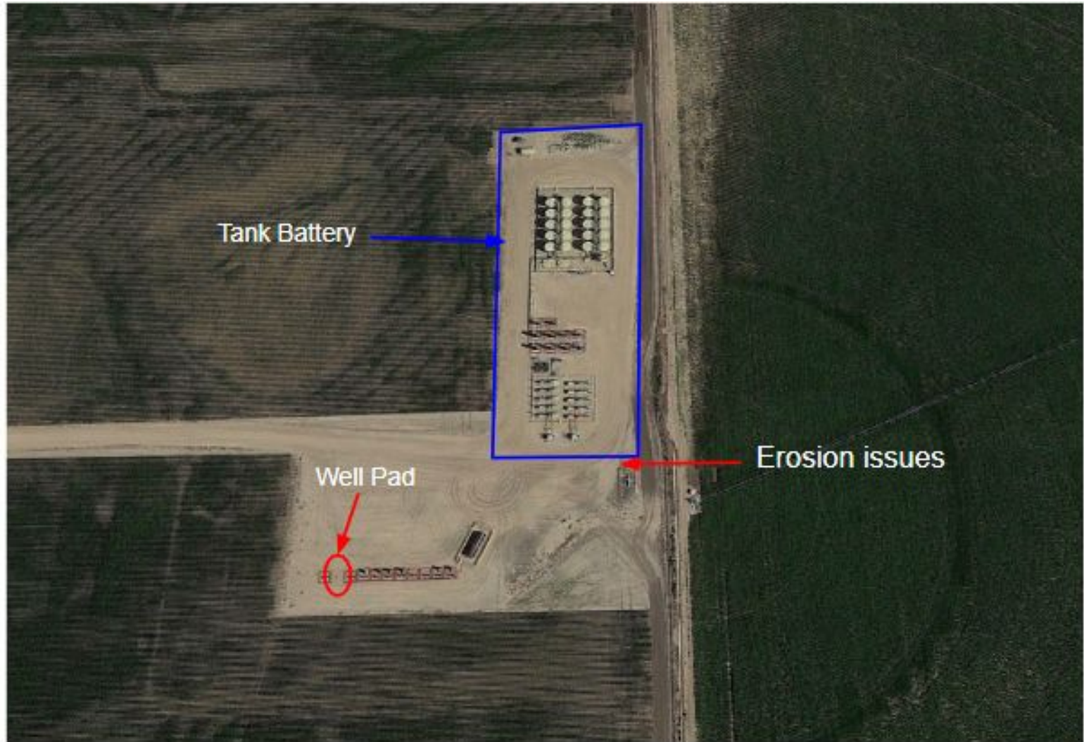
Photo 1. 2021 aerial imagery of the well pad (north is up). The tank battery (highlighted in blue) remains to service the producing wells on site. Note: rill erosion location.
