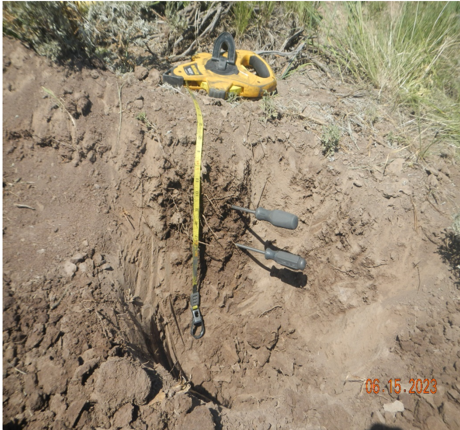
Photo 9. View of test hole for topsoil evaluation.
