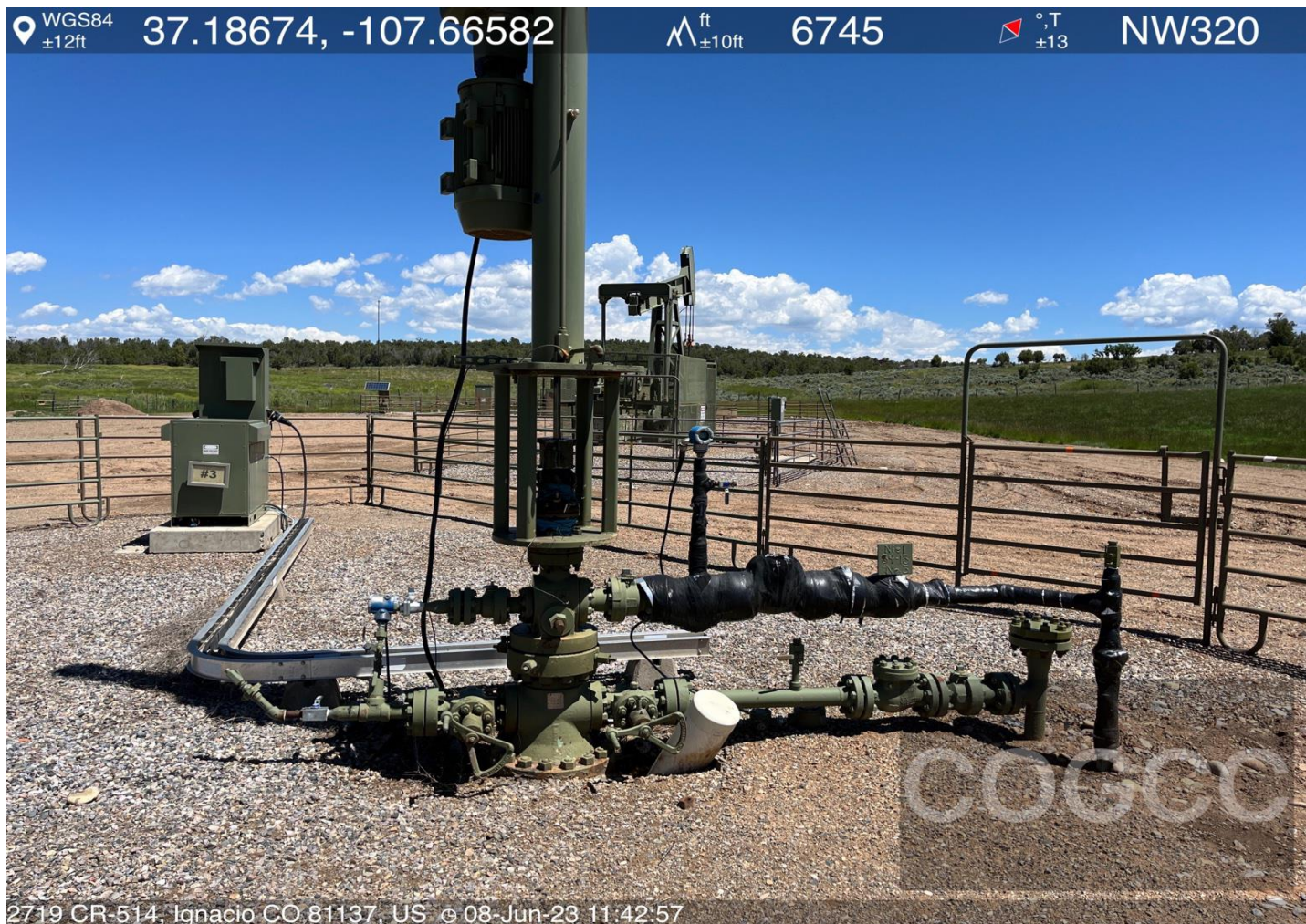
Photo #3. View of the #3 wellhead assembly.
