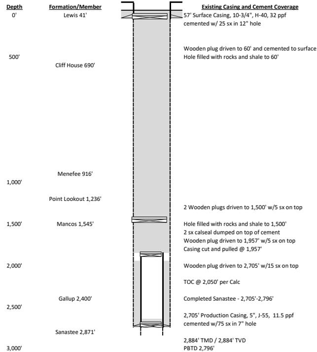
\*BOP or other mechanical method should be used for well control
